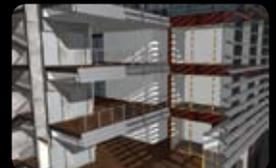
**Model-based version tracking** - For best in class coordination workflow with Engineers, ArchiCAD 14 allows architects to compare IFC model versions and to import only differences, displaying design changes with color codes in the architectural model context.
