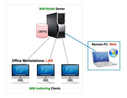
To enable individual clients to work on their part of the BIM model requires that the model can be managed as discrete parts. To achieve this, within the BIM model parts need to be granulated at the level of "atomic" elements (building components) and stored as database records on the server. In addition it is essential that integrity of element relationships and their structure within the BIM model is maintained.
