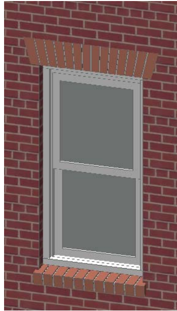
Masonry Jack Arch
