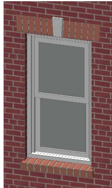
Masonry Jack Arch with Keystone
